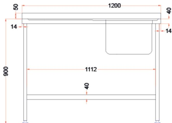
The fully welded 1200mm wide sink from Holmes is made from commercial grade stainless steel, and features a left side drainer with right side bowl. The 304 stainless steel is highly resistant to rusting and stains, as well as smooth and easy to clean which makes it ideal for use in commercial kitchens. The sink allows you to create practical and hygienic washing areas in your kitchens, and features a strong, sturdy undershelf for the additional storage of supplies and utensils.
